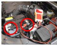
1. Connect the gas tube with car air intake or air filter. Connect wireless transmitter. Start car.
