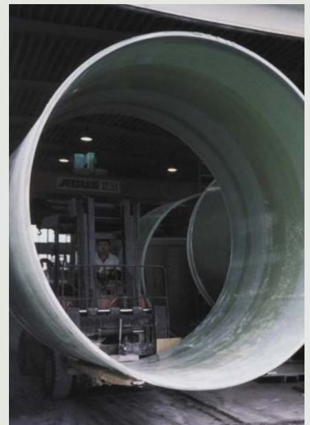
GRP cylinder · Diameter 9.9 ft.
