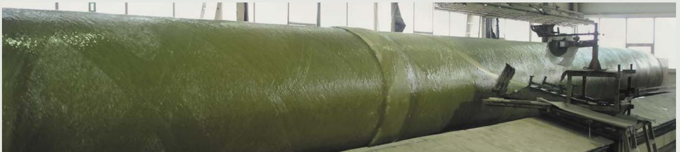
Filament winding at IBK-Fibertec using a mandrel with a diameter of 5.25 ft. and a length of 72.2 ft.
