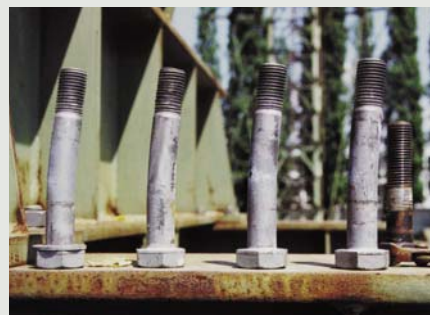
Twisted bolts yet before the cylinder could be crashed
