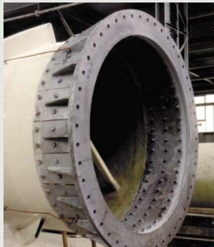
External steel flange
