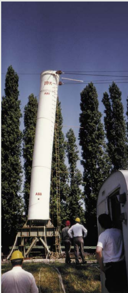
Crash test with a GRP cylinder
